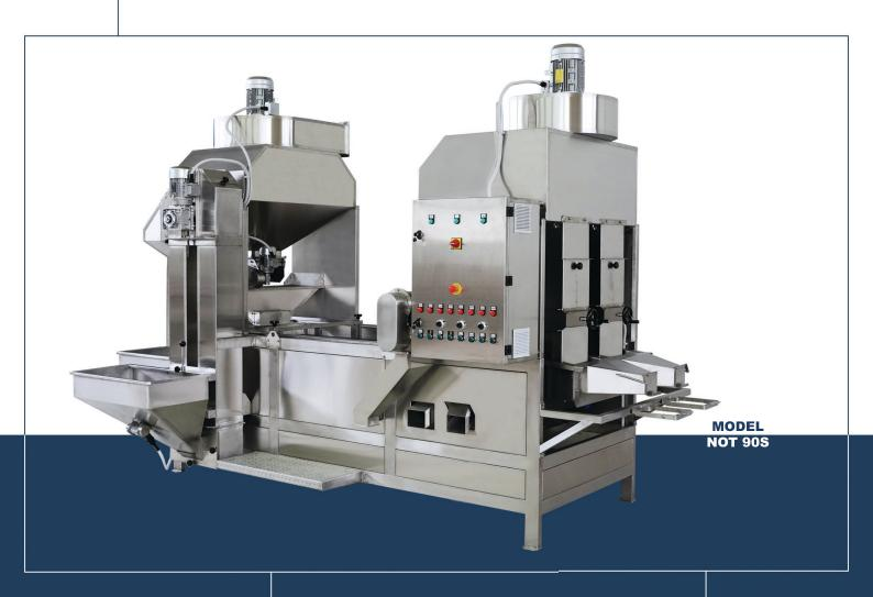
NOT 90S is a dry nuts cleaning and sorting machine. It has all the technical specifications and standards of modern and innovative production unit. It has a rapid production times and complies with food hyegin and safety regulations.
