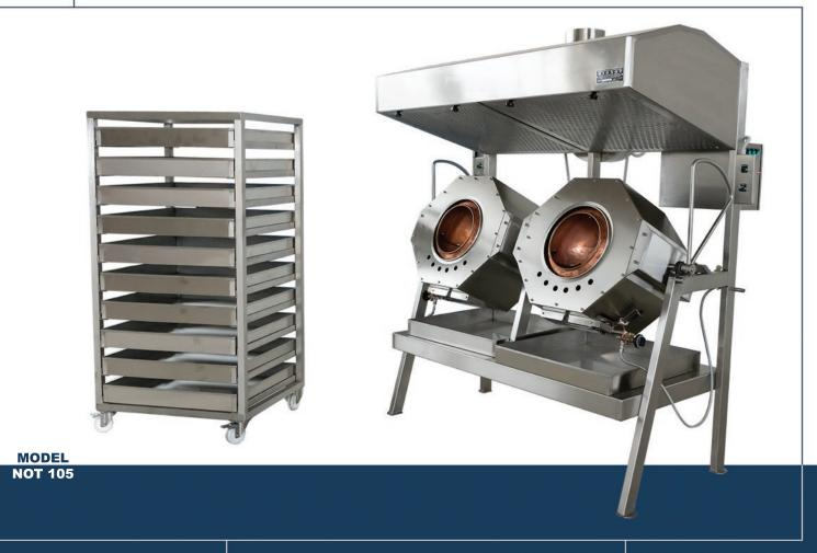
The model NOT 105, is an quick and easy solution for the production of caramel coated nuts. The processing of the nuts is performed inside two rotating drums, where nuts and coatting material are inserted.
