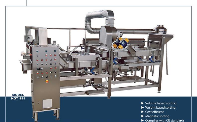
BIONOT sorting and cleaning machines for nuts and seeds are made entirely of stainless steel and meet all the standards of modern industry as well as international norms for hygiene and food safety. They can be manufactured for varius production flows so they can be used in both small and big industries.
