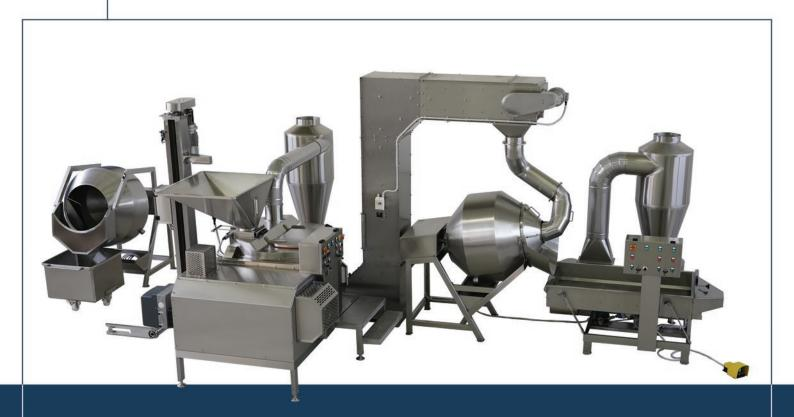
Coating nuts is a very specialized processing procedure with specific demands. The know-how as well as the most appropriate selection of systems are vital for achieving a qualitative result. This frying-coating line of BIONOT response to this specific requirements with a complete semi-automated system of advance technology, in which human presence is not required at all stages.
