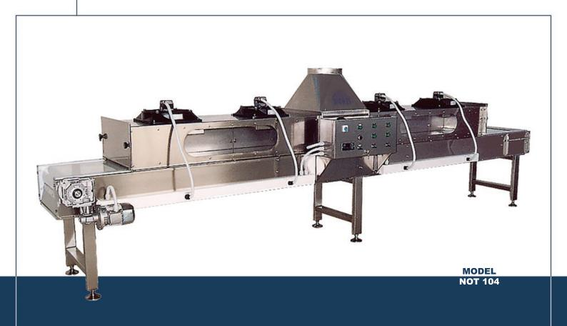
The model NOT 104 is a cooling tunnel for caramelized nuts, sesame bars and similar products. It can be manufactured for various production sizes and applications.
