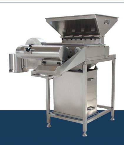
The model SRB is a machine that removes red skin from peanuts. It is equipped with a suction system for transferring the red skins to a special collector for their disposal.
